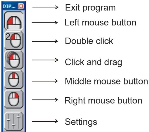
Each pushbutton is assigned to a mouse button. By resting the mouse pointer on a certain pushbutton, either a new action can be preselected, or the current action can be switched off.
